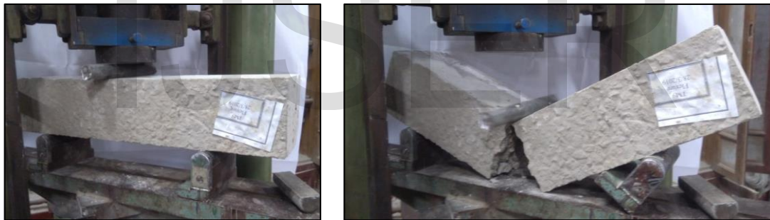
Figure 3: The Performed Flexure Test.
