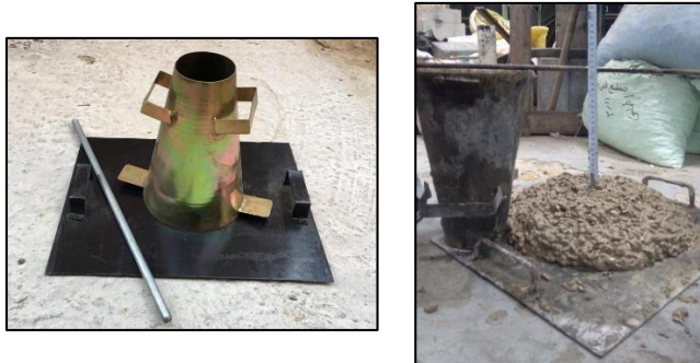
Figure 1: The Performed Slump Test.
