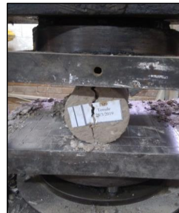
Figure 4: The Performed Splitting Tensile Strength Test.
